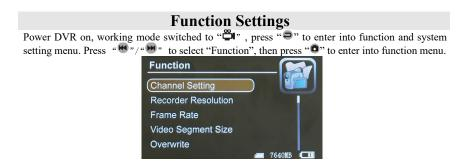
1. Channel Setting: Press "♥" / "♥" to select "Channel Setting", and then press "♥" to enter. Press "♥" / "♥" to select "A,B,C,D" then press "♥" to select and exit.
